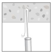
Clear hole of drilling debris.
