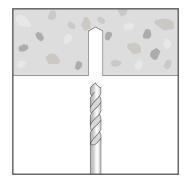
Drill hole into substrate to the specified diameter and depth.
