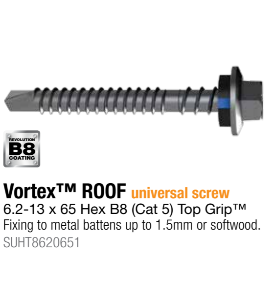
Region D Vortex 6.2-13 x 65 Hex B8 (Cat 5) Fixing to softwood and metal battens up to 1.5mm in high wind areas. SUHC862065R
