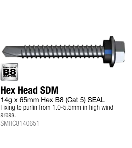
Region D SDM 14g x 65mm Hex B8 (Cat 5) Fixing to purlin from 1.0-5.5mm in high wind areas. SMHC814065R
