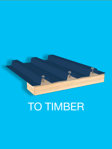
Hex Head Type 17 14g x 65mm Hex B8 (Cat 5) SEAL Fixing to softwood or hardwood in high wind areas. STHC8140651
