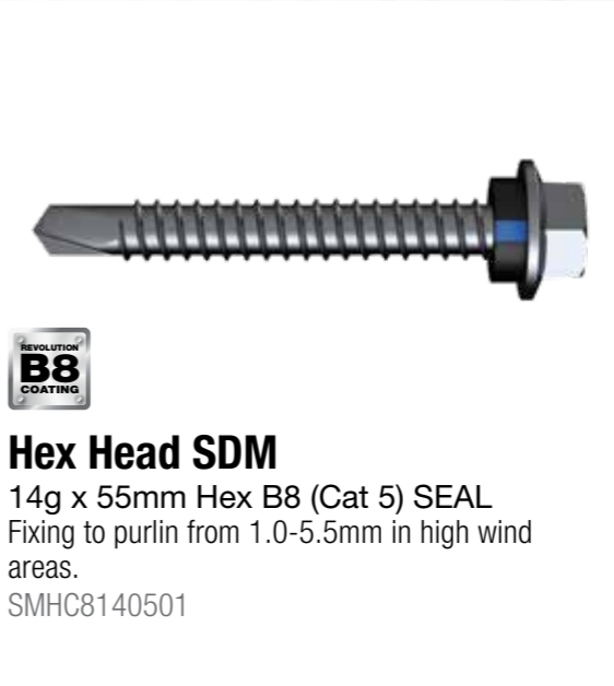
Region D SDM 14-10 x 55 Hex B8 (Cat 5) Fixing to purlin from 1.0-5.5mm in high wind areas. SMHC814055R
