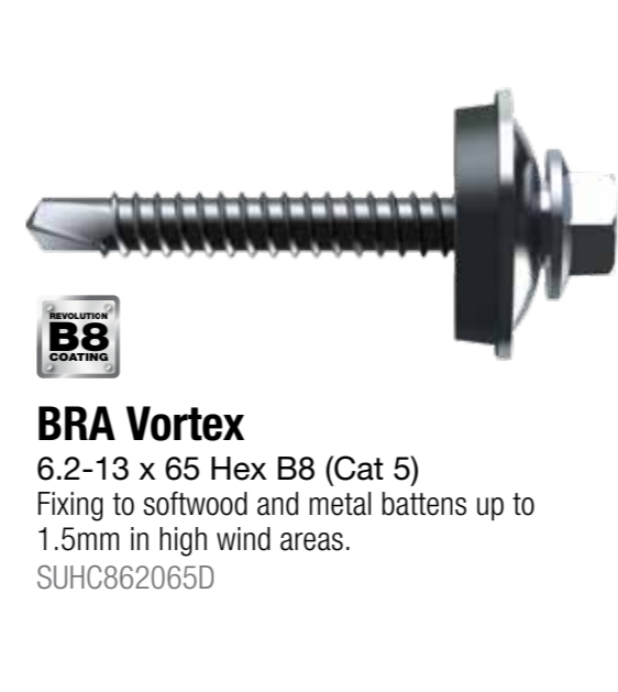
Region D Vortex 6.2-13 x 65 Hex B8 (Cat 5) Fixing to softwood and metal battens up to 1.5mm in high wind areas. SUHC862065R
