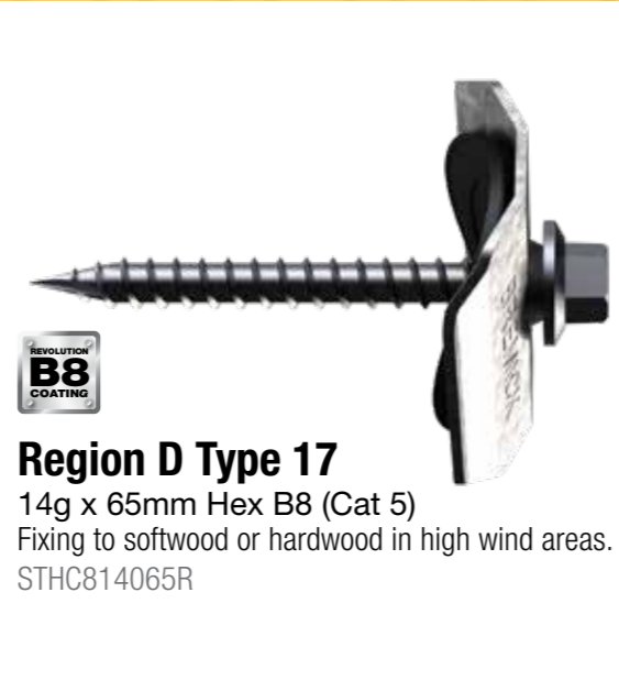
Hex Head Type 17 14g x 65mm Hex B8 (Cat 5) SEAL Fixing to softwood or hardwood in high wind areas. STHC8140651
