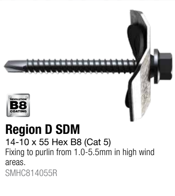
Hex Head SDM 14g x 55mm Hex B8 (Cat 5) SEAL Fixing to purlin from 1.0-5.5mm in high wind areas. SMHC8140501
