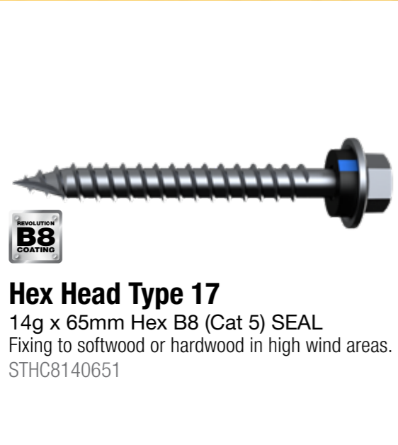
Region D Type 17 14g x 65mm Hex B8 (Cat 5) Fixing to softwood or hardwood in high wind areas. STHC814065R
