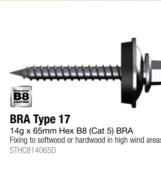
Region D Type 17 14g x 65mm Hex B8 (Cat 5) Fixing to softwood or hardwood in high wind areas. STHC814065R
